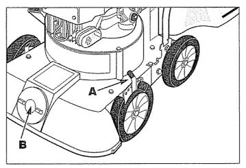
Figure 5: Vacuum Height Adjustment Lever and Inlet Cap.
